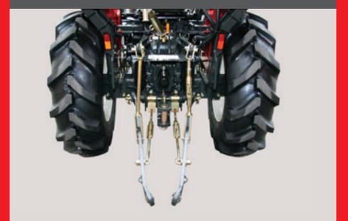
3-point hitch rear Category I provides a lift capacity of 650 kg.
