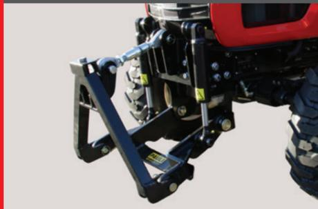
Frontlift cat. 0 with a lift capacity of 700 kg.
