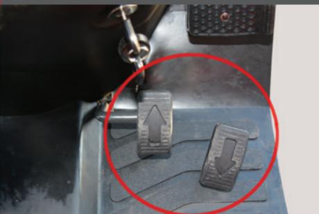
Hydrostatic control pedals for smooth handsfree forward & reverse motion (hst-models).
