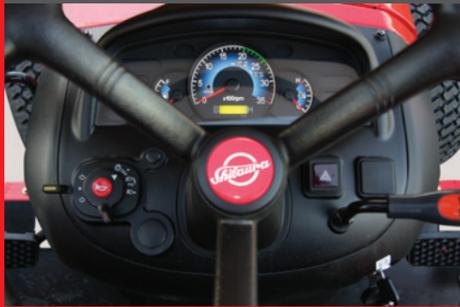
Clear visibility of dashboard allows easy monitoring of the tractor's condition: rated speed, temperature and tank capacity.
