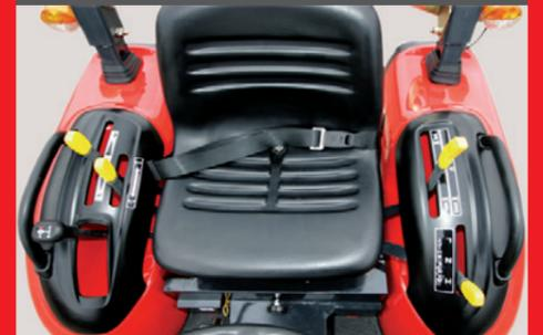
The operating levers are placed within easy reach on the left and right of the seat for ergonomic operation.
